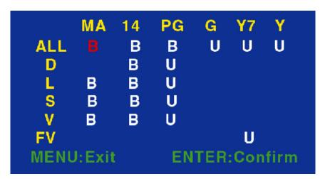
Select **TV Rating Guide** to set rating grade. Use remote control arrow keys to move cursor to desire rating grade. When the text turns red, press **ENTER** key to set block **(B)** or unblock **(U)** condition.
